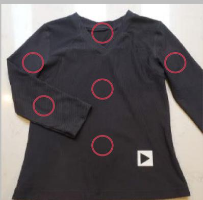
Figure 1. MSG with highlighted circles indicating IMU locations
