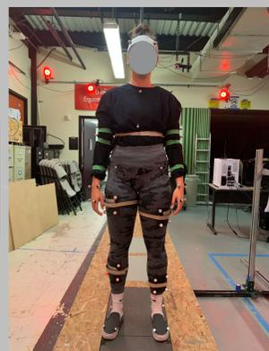
Figure 2. Retroreflective markers were placed based on a modified Helen Hayes full body marker set.
