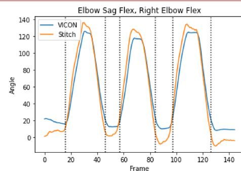
Figure 3. Processed angles showing VICON data relative to Stitch data for three cycles of elbow sagittal flexion of the right elbow in the flexion direction. Dotted lines denote cycles.
